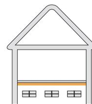
When installed above "occupied spaces", such as workshops, garages, and basements, a suitable compliant lining such as plasterboard or fibre cement should be installed over the insulation. Alternatively, we recommend installing **ecoinsulation Faced Thermal underfloor**.
